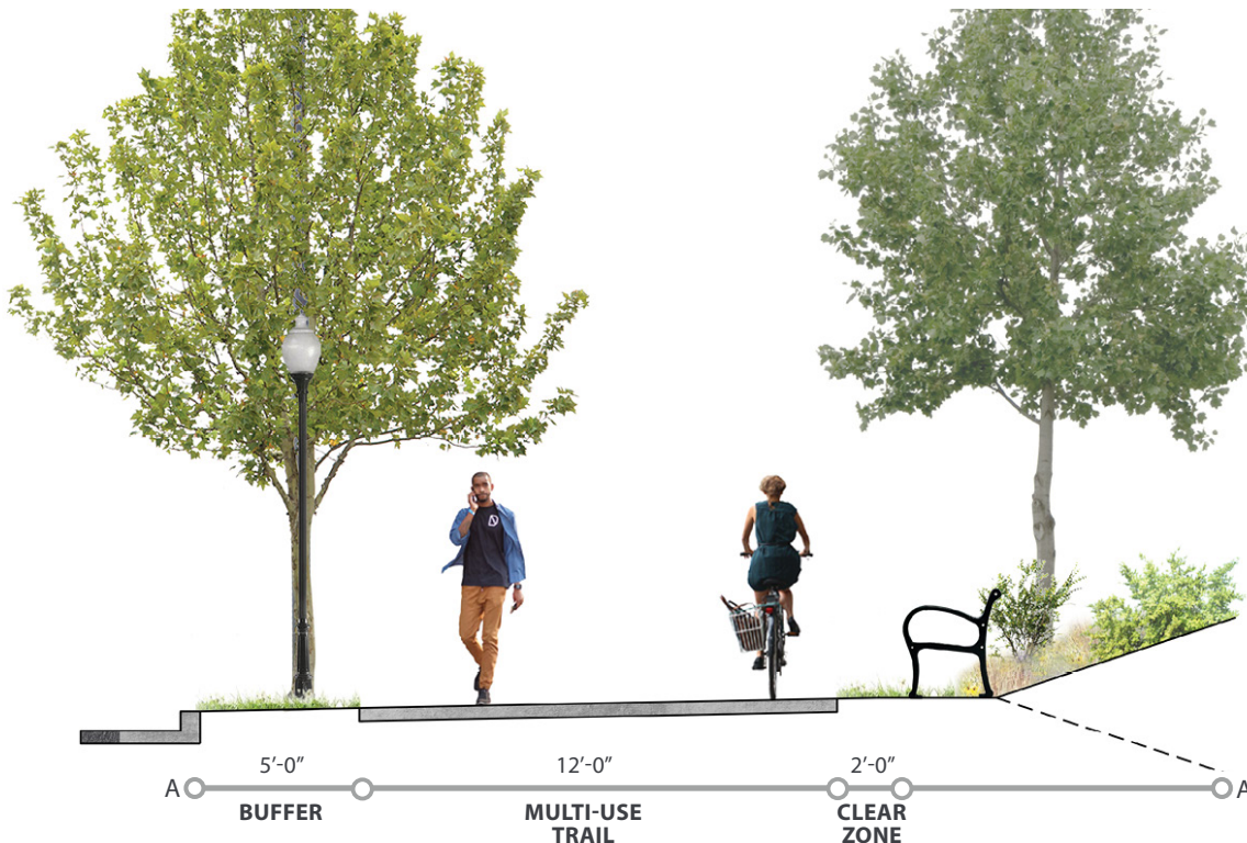
This cross-section depicts a typical on-road trail.
