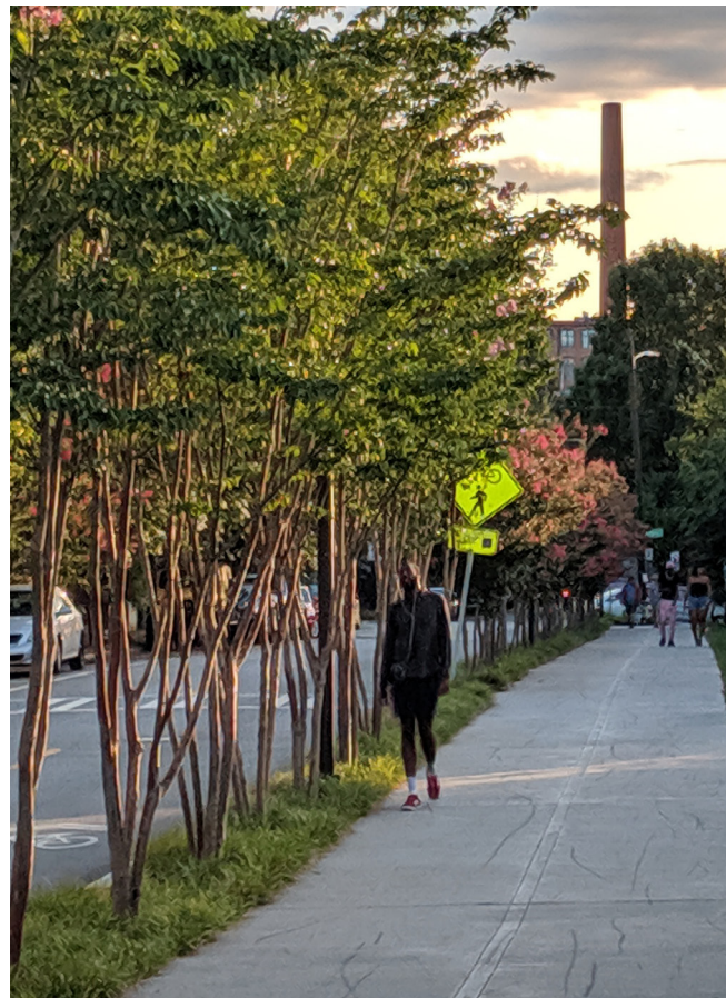
An example of pedestrian-vehicular separation using a tree-lined landscape strip.
